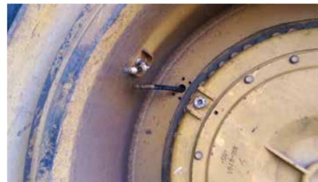
*Before: Position 3 and 6 double gutter wheel on the 789, the valve stem was prone to damage from rocks and debris, causing the tyre to deflate*
